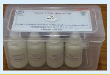
CIBA-CMH Mineral kit - A portable kit developed by CIBA can estimate the amount of Calcium, Magnesium and Hardness in pond waters of all salinities, with minimal volume of water sample and 95% accuracy at field level. The kit has higher shelf life of the reagents and easy to use.
