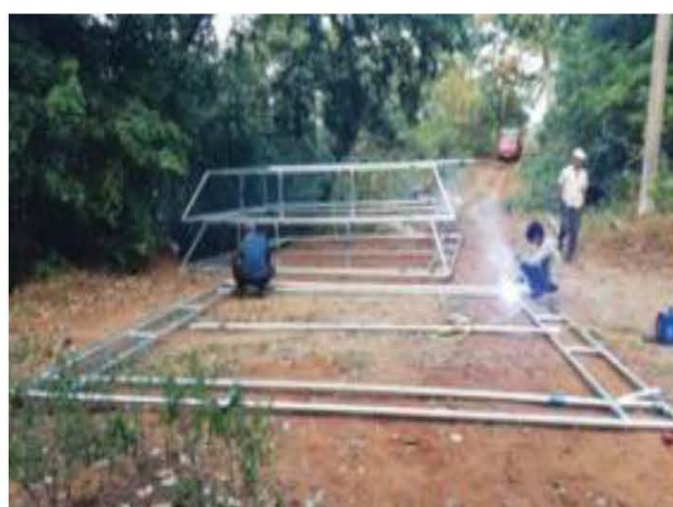
GI pipes cutting and welding for fabrication of cage frames
