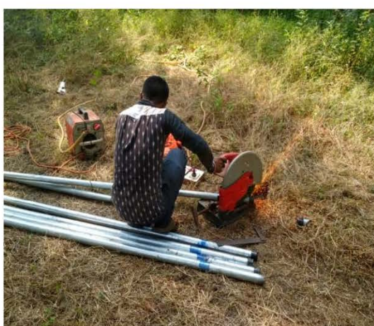
GI pipes cutting and welding for fabrication of cage frames
