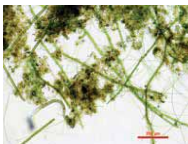
Microscopic view of the floc generated in the FWH supplemented treatments
