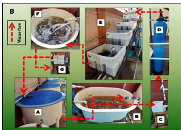
A. RAS with tubing bioreactor, B. RAS with raceway type bioreactor, C. RAS with rotating wheel bioreactor. Components: a. shrimp culture tanks, b. Sump, c. pump, d. pressure sand filter, e. seaweed bioreactor, f. collection tank, g. circulating pump
