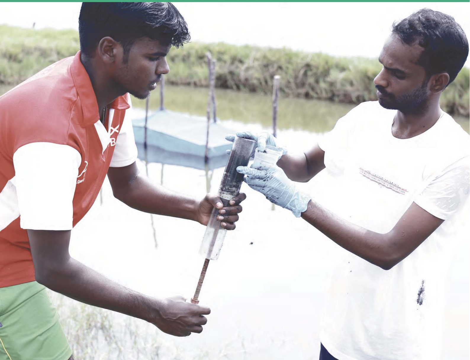
Sampling of soil for profiling of minerals in aquaculture ponds
