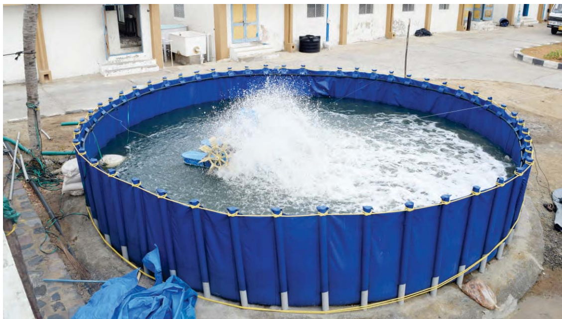
Efficiency of aeration was evaluated in special experimental tank system built in Muttukadu Experimental Station
