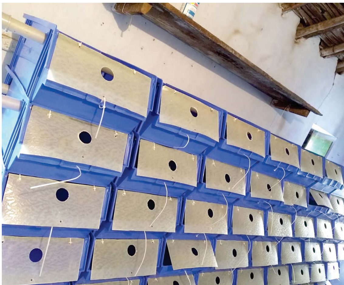
RAS based indoor system for mud crab rearing using formulated feed Scylla Plus
