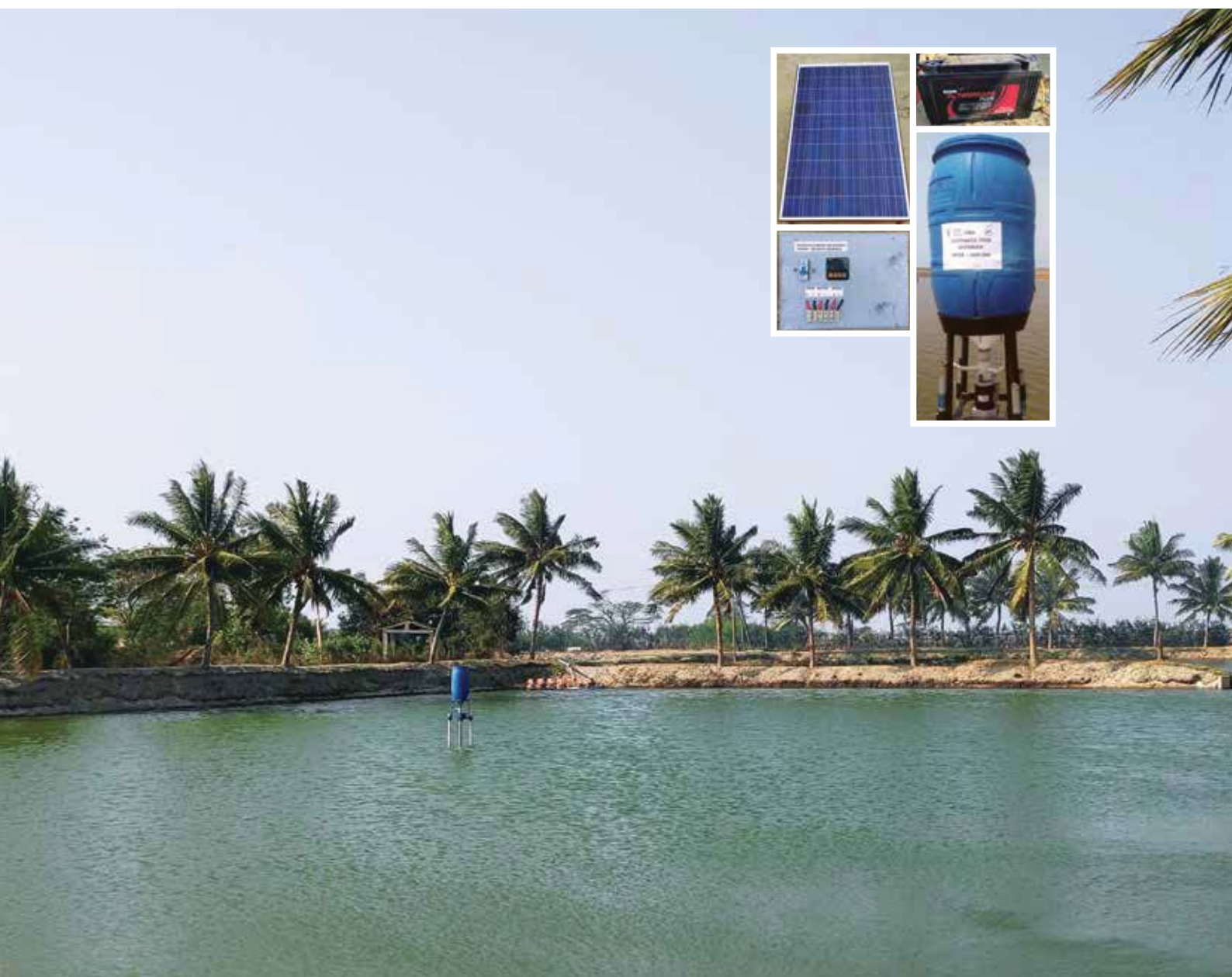
Solar based Autofeeder installed in farmer's pond
